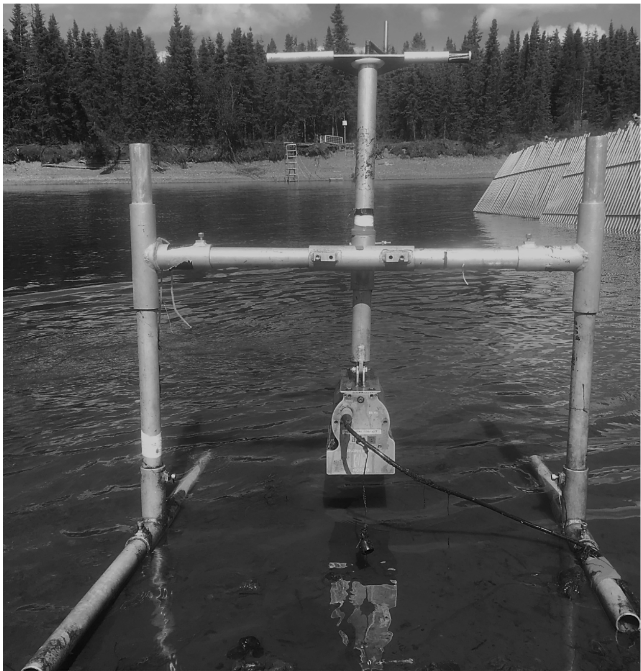
Figure 6.—View of a DIDSON mounted to aluminum H-mount with manual crank-style rotator at the Anvik River sonar project, 2018. Photo taken 2017.
